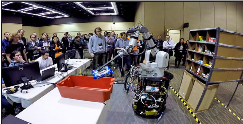
Figure 1: The RBO team's robot placing a pack of Oreo cookies that it retrieved from the warehouse shelf into a tote. Image courtesy of RBO team.
